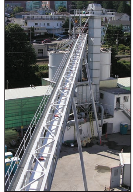
Aeration conveyor being fed by bucket elevator.
