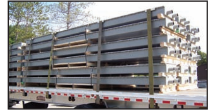
Aerated troughs for dome floor installation.
